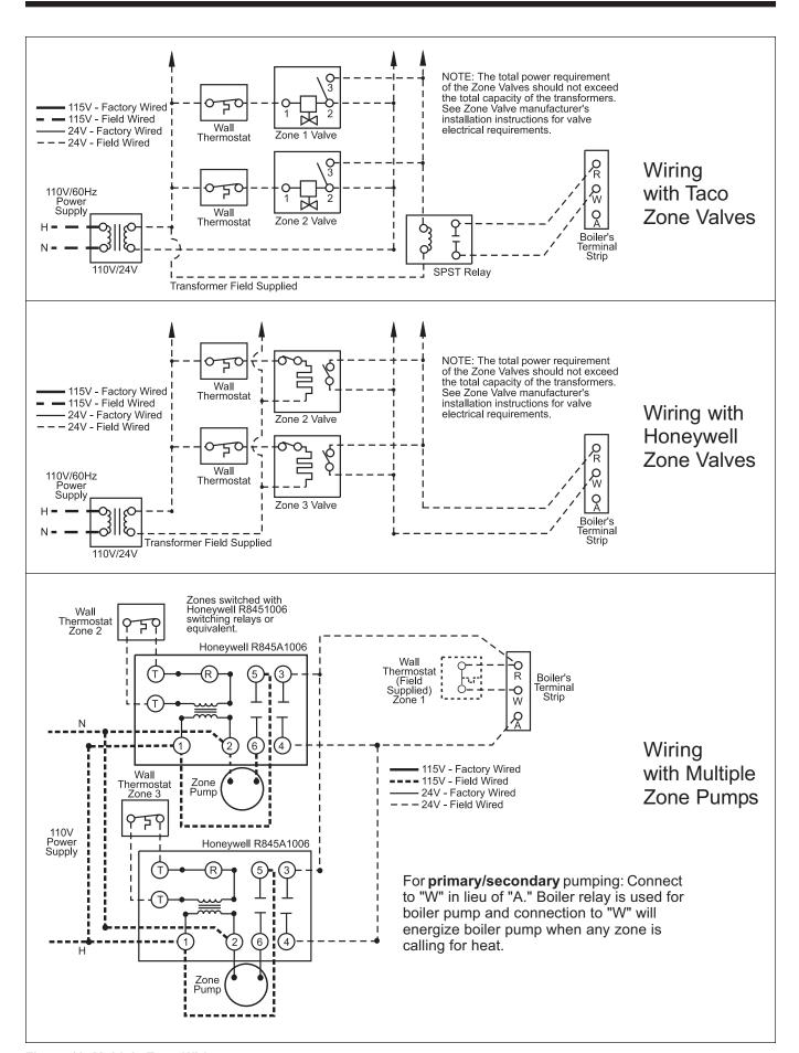
Figure 10. Multiple Zone Wiring.
